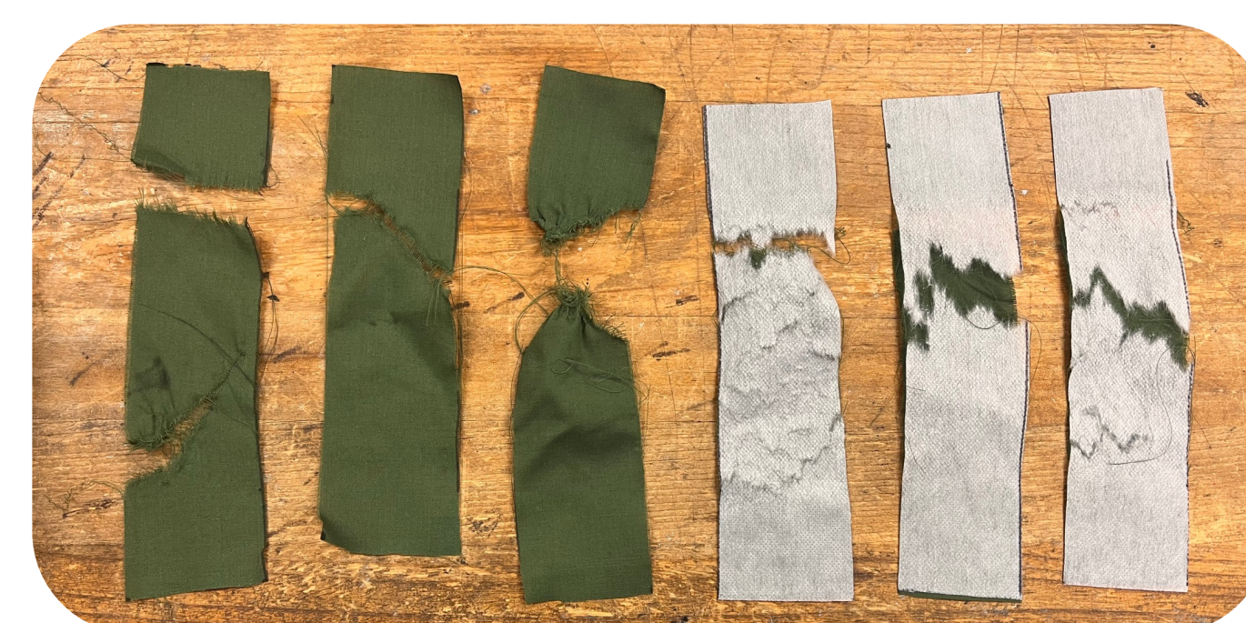
Fig. 6: Tensile and shear tests were performed on fabric and hook-and-loop components to inform the amount of fabric used in the design
