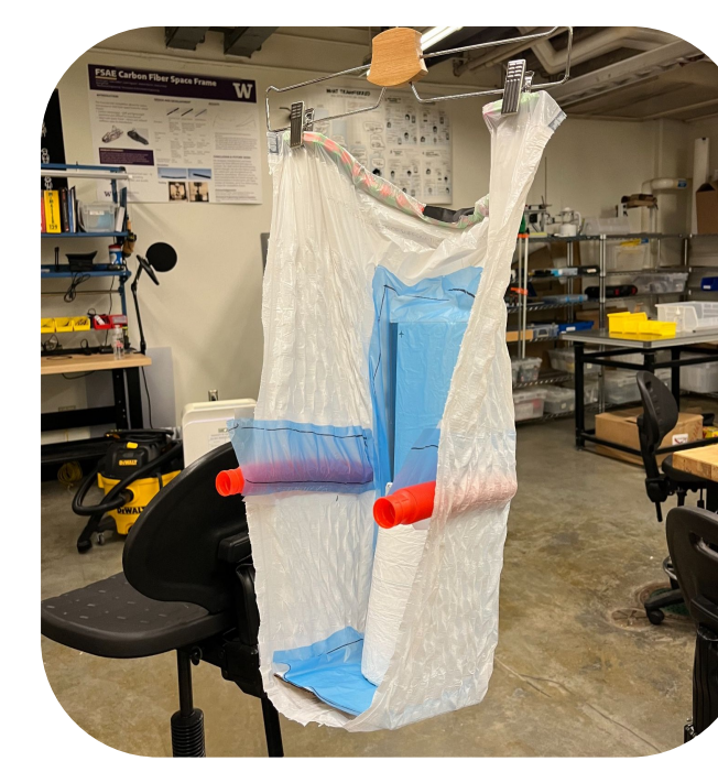
Fig. 3: Chair scale modeling to test stiff inserts and arm rests
